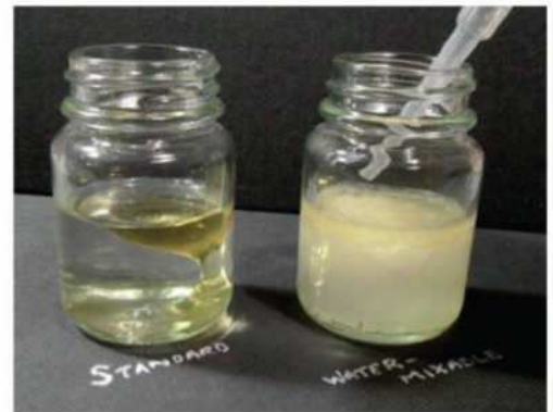
By adding an emulsifier to the oil, water easily mixes with the oil molecules.
